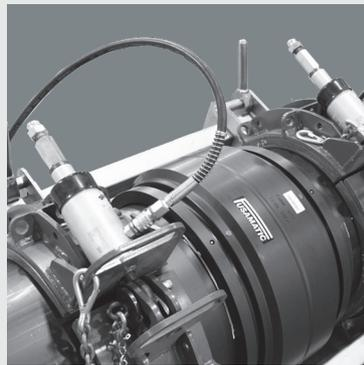
**14.** The pipe should not be subjected to bending loads or sagging during the assembly process. Position the pipe so that it is not under any stress and ensure the pipe or fitting is supported underneath.
