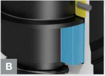
If the valve is over torqued during opening or closing, the connector is designed to fail before the valve seals, thus preventing a leak to atmosphere. The **safety connector** can be replaced under live conditions
