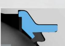
The **seat retainer** design ensures the ball seat is kept in place at all times. This optimal design prevents the ball seat from being dislodged, which guarantees a good functionality throughout the years.
