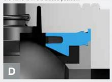
The **seat retainer and support ring** design ensure the ball seat is kept in place at all times. This optimal design prevents the ball seat from being dislodged, which guarantees a good functionality throughout the years.
