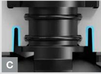
The flexible spindle shaft ensures equal compression around the O-rings when loaded by internal pressure. At the same time the groove will adapt to any deformation as a result of upstream pressure on the ball when the valve is in the closed position
